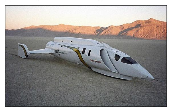
The car has been rebuilt and re-wired from the ground up with a longer wheelbase, wider track and modified aerodynamics, including lengthened wheel covers and parachute assembly and no dorsal fin. The braking parachute and its deployment system were also completely re-designed.
