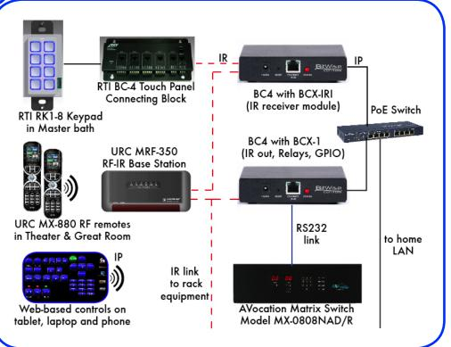
**Control interfaces** – URC MX880 RF remotes were ideal for the theater and great room, with both communicating to an MRF350 unit in the rack. In the master bath an RTI keypad connected to their CB-4 unit. Finally a web interface was used to bring a tablet, laptop and iPhone into play. The MRF350 and CB-4 base-units both communicated with a second BC4 via an IR Reciever.
